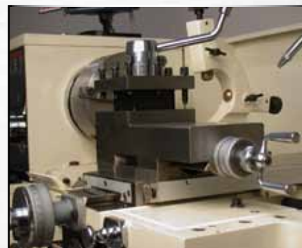
Every JET ZX Lathe Comes with a Four-Way Tool Post
