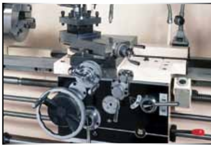
Carriage Features One-Shot Lubrication and Turcite B on Sliding Surfaces
