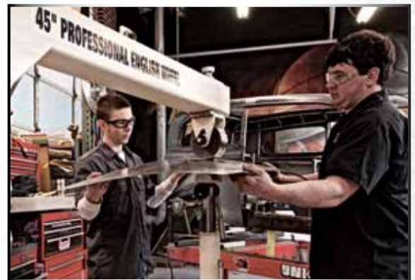
45" Deep Throat Depth Makes it Easy to Work with Large Panels
