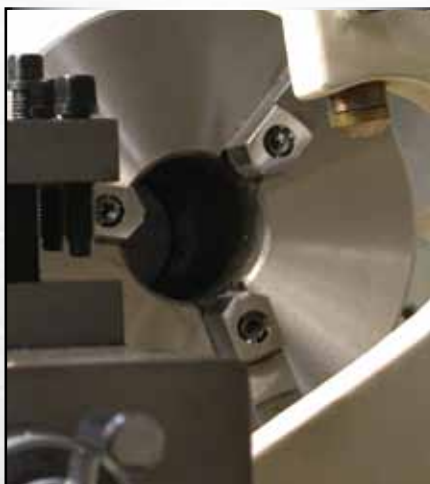
Large 3-1/8" Spindle Bore
